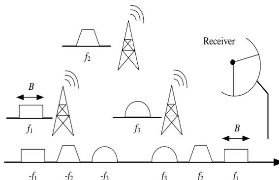
**Fig 1.** Three RF transmissions with different carriers  $f_i$ . The receiver sees a multiband signal.
