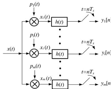
**Fig 2.** The modulated wideband converter-a practical sampling stage for multiband signals
